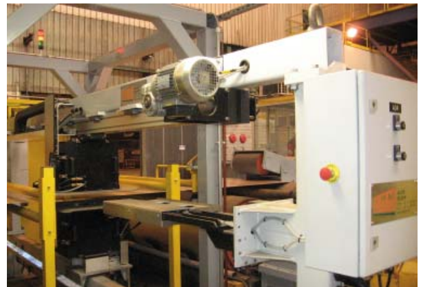
The FVXR-1 coating weight gauge on site.
